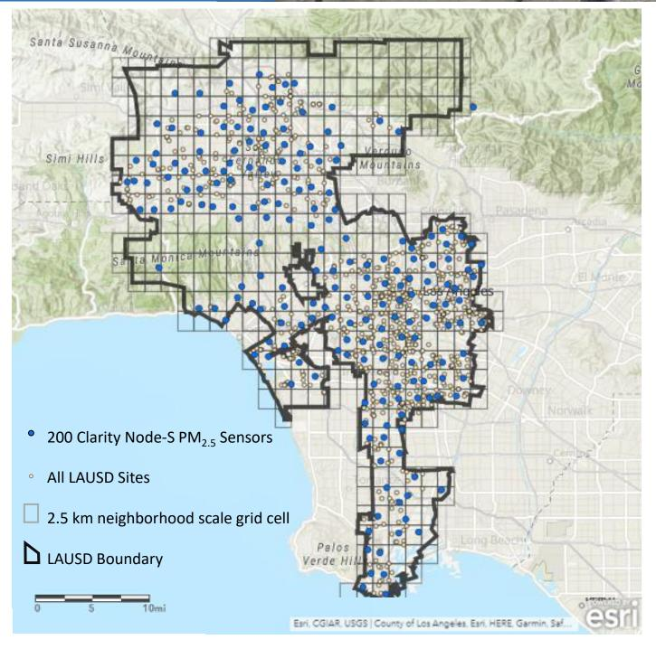
The Los Angeles Unified Know Your Air Network includes 202 Clarity Node-S devices. The network is a "neighborhood scale" design, which outlines a uniform grid of 2.5 kilometer (~1.6 mile) squares. The sensors are deployed so that one is at or near every school within Los Angeles Unified.
